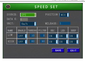
• **Source**: GPS/Vehicle, if choose "vehicle', speed pulse signal should be connected.
