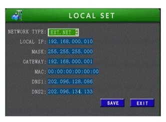
Setting of local IP, you can connect to RJ45 to Ethernet.
