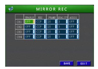
**Enable**: **ON**: Turning on the channel; **OFF**: the channel will not record video and the log will not be lost even video is lost
