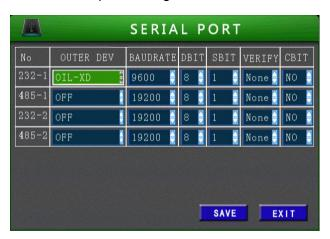
Select external equipment at serial ports and parameters as baud rate will be default. If the external parameters dis-accord from default ones, you can modify them manually and save them before you exit.
