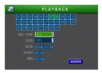
Calendar: Green means normal video recorded, red means alarming video recorded and blank means no video recorded.
